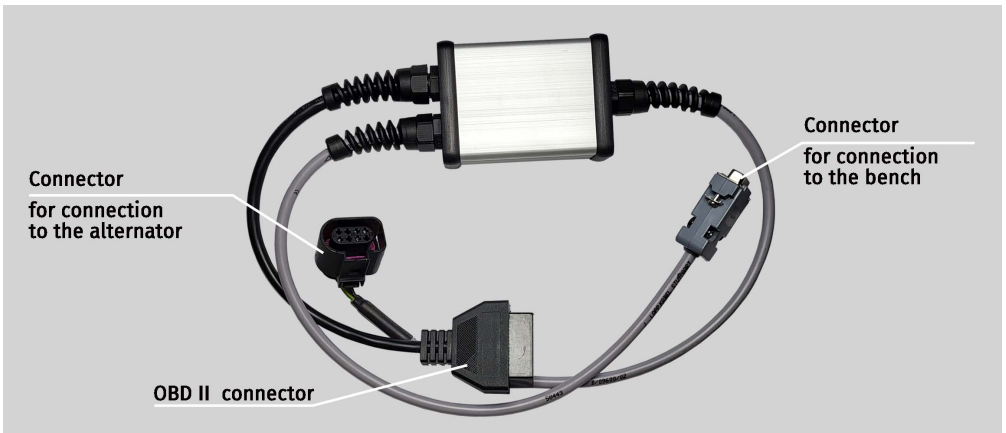
Figure 8. Cable for testing 48 V belt starter-generators
